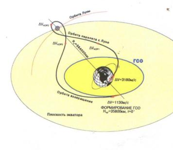
Translunar opens way to undetected access to GPS (12-hr), GEO, retro-GEO, unexpected low-altitude passes, etc. 55
