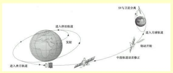
Typical trajectory of simple lunar probe shows checkout, transfer, and arrival.
