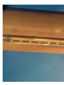
RETURN TO FRIGHT: GAPS IN THE INSULATION FOAM ON DISCOVERY'S EXTERNAL TANK SHOW FOAM LOSS FROM THE TANK'S PROTUBERANCE AIR LOAD (PAL) RAMP. A FOAM IMPACT LED TO THE DESTRUCTION OF THE COLUMBIA SHUTTLE DURING RE-ENTRY ON FEBRUARY 1, 2003. Image Credit: NASA
