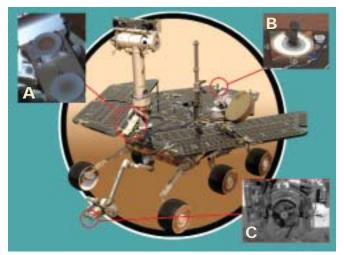
The mast assembly acts as a periscope for the spectrometer science instrument that is housed inside the Rover body, and it provides height and a better point of view for the Panoramic Cameras and the Navigation Cameras. Motors can turn the cameras full circle, or tilt them straight up or down. Details: (A) dust collection magnets, (B) color calibration sheets with sundial (provided by Planetary Society) and (C) rock abrasion tool.
